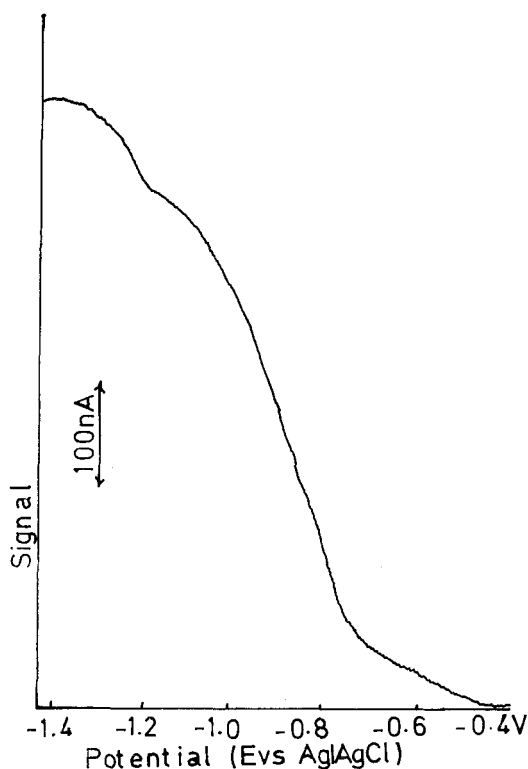
FIGURE 1 DC-Polarogram of butorphanol tartrate (1mg/30ml) in an alkaline medium. Damping=2.
